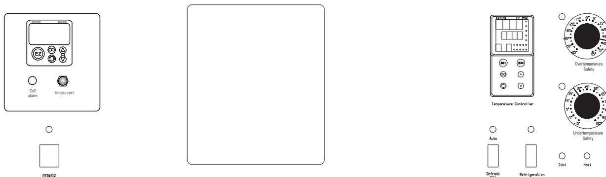
**Figure 2-1.** Environmental Chamber Control Panel (shown with optional CO<sub>2</sub> control)
